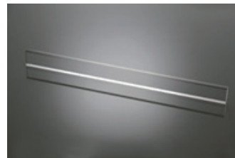
Quartz rod (Dimension, 447x34x14 mm; end flatness, < \lambda/4 @ 632.8 nm; side flatness < 40\lambda @ 632.8 nm), a crucial optical element required for lithography illumination system.
