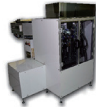
Development of 12-inch PEALD system in ITRC for the purpose of depositing ultra-thin film ( < 20 nm) with a high step-coverage over high aspect-ratio trench.
