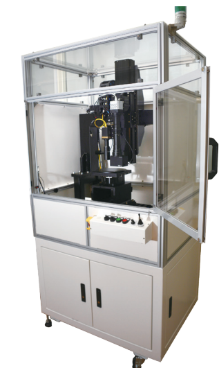
High-resolution automated optical testing device for LED chip defects The device is projected to replace the current manual testing methods and capable of testing 4" LED wafer chip defects within 20 minutes. This would further enhance the competitiveness of Taiwan's LED industry.
