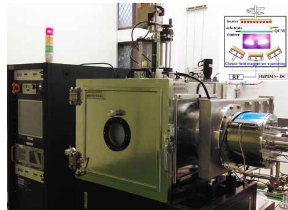
The new sputtering technology developed by ITRC can be applied to sputter high-hardness thin films and DUV fluoride thin films.
