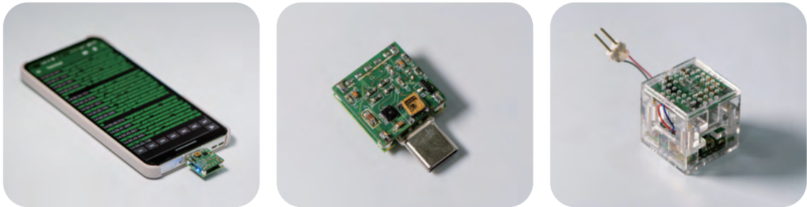
具即時溫/濕度補償功能、藍牙通訊與有線通訊氣體感測器元件公板模組 Gas sensor component CRB modules with real-time temperature/humidity compensation function, Bluetooth, and wired communication.
